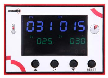
The central controller allows for setting the desired temperature (° C and ° F), as well as the press duration in seconds. The green digits because represent the target values, while the white numbers reflect the current values. The counter is displayed at the lower right and indicates the number of pressing operations carried out since the last reset.
