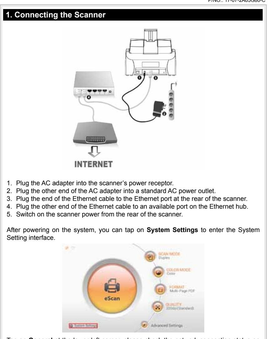
1. Plug the AC adapter into the scanner's power receptacle.
