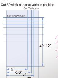
Internal vertical slitter moves at 4 positions.
